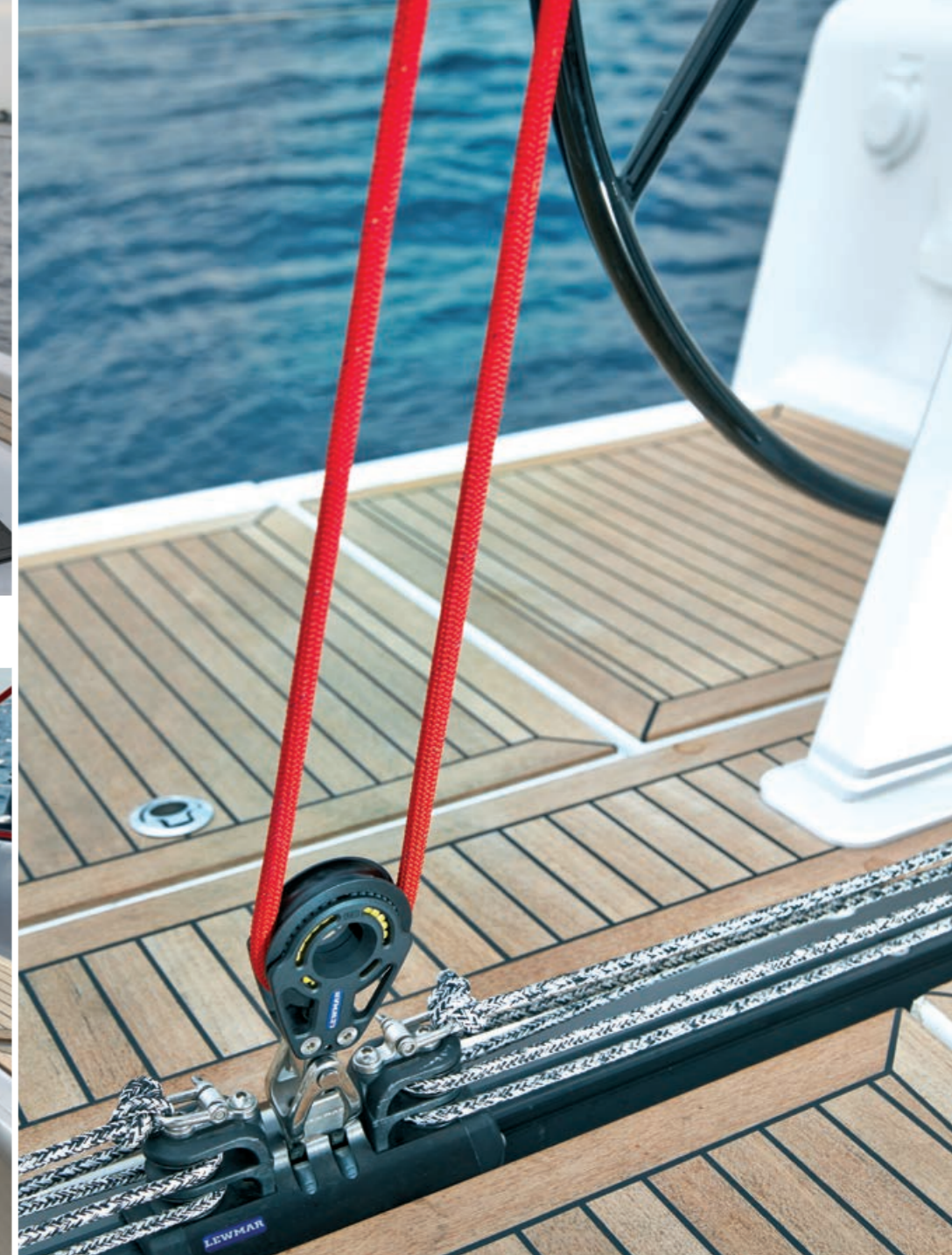
Being recessed into the floor, the mainsheet traveller allows an ideal trim of the mainsail.
